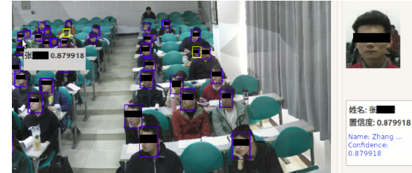
Figure 3: The main user interface of the NaMemo System. The rectangles frame the recognized students. The blue ones indicate confidence levels above 0.8, while that in the yellow ones are below 0.8 and over 0.5. When the cursor is located in a frame area, the teacher could see the student's profile on the right part of the window. The blue text is the translation.
